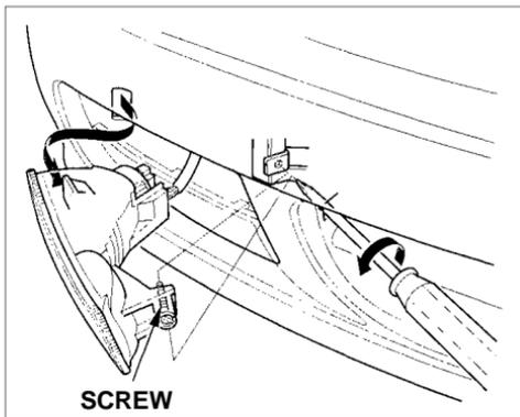
1. Use a Phillips-head screwdriver to loosen the turn signal assembly's mounting screw.
