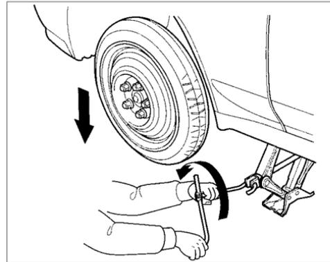
14. Lower the vehicle to the ground and remove the jack.
