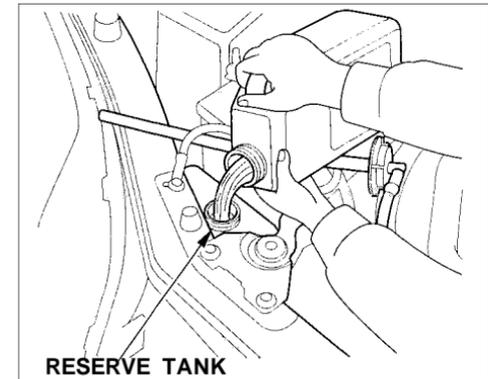
10. Turn off the engine. Check the level in the radiator, add coolant if needed. Install the radiator cap, and tighten it fully.
