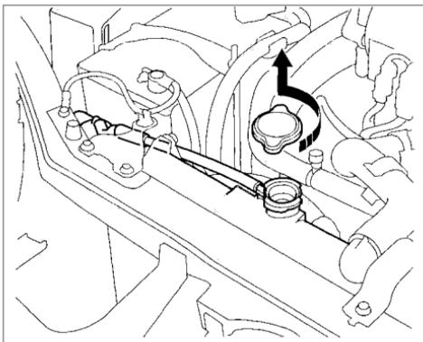
1. Slide the heater temperature control lever to maximum heat. Open the hood. Make sure the engine and radiator are cool to the touch.
