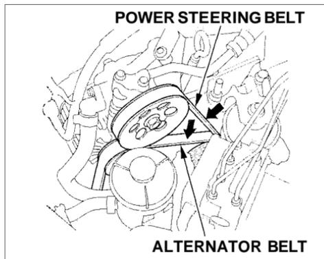
Check the condition of the two drive belts. Examine the edges of each belt for cracks or fraying. Check the tension of each belt by pushing on it with your thumb midway between the pulleys.
