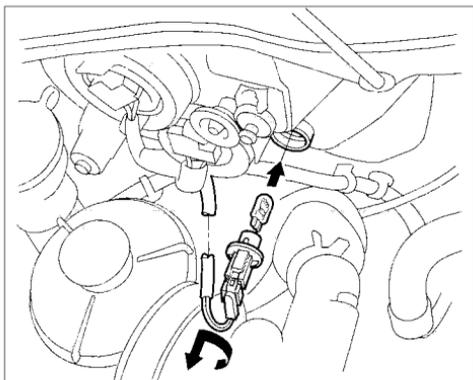
2. Remove the socket from the headlight assembly by turning it one-quarter turn counterclockwise.
