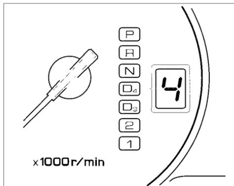
This indicator in the tachometer shows which position the shift lever is in. The illuminated number next to the "D4" indicator shows you the gear you have selected in the Sequential SportShift mode.
