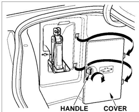
6. The jack is behind a cover in the left fender. Remove the cover by turning the handle clockwise, then pulling on the cover.
