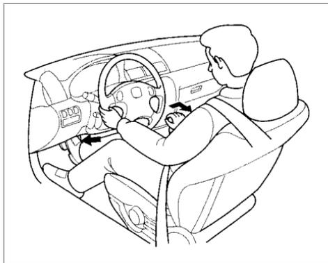
To avoid transmission damage, come to a complete stop before shifting into Park. The shift lever must be in Park before you can remove the key from the ignition switch.
