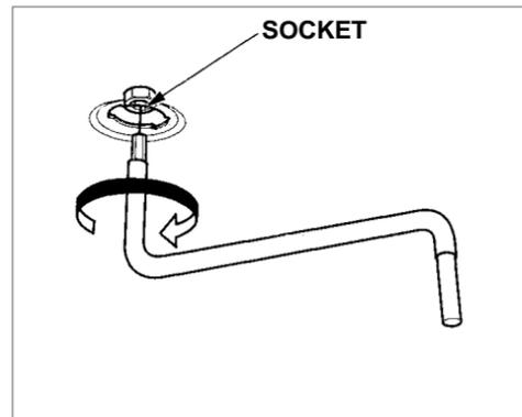
5. Insert the moonroof wrench into the socket behind this plug. Turn the wrench until the moonroof is fully closed.
