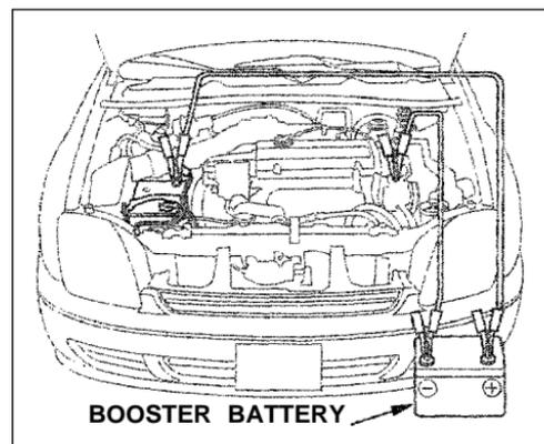
6. Start your vehicle. If the starter motor still operates slowly, check the jumper cable connections to make sure they have good metal-to-metal contact.
