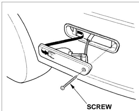
1. Use a Phillips-head screwdriver to remove the side marker assembly's mounting screw.
