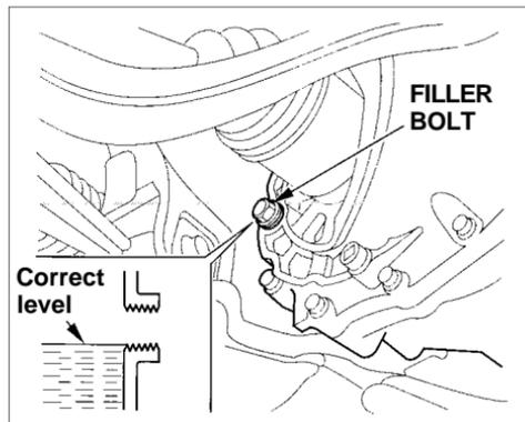
Check the fluid level with the transmission at normal operating temperature and the vehicle sitting on level ground. Remove the transmission filler bolt and carefully feel inside the bolt hole with your finger. The fluid level should be up to the edge of the bolt hole. If it is not, add Genuine Honda Manual Transmission Fluid (MTF) until it starts to run out of the hole. Reinstall the filler bolt and tighten it securely.
