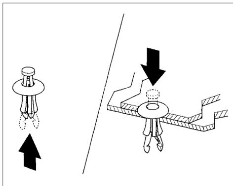
9. Reset the fastener by pushing on the pointed end until it pops back almost flush with the fingers on the housing.
