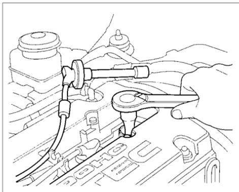
6. Torque the spark plug. (If you do not have a torque wrench, tighten the spark plug two-thirds of a turn after it contacts the cylinder head.)
