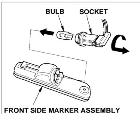
3. Remove the socket from the side marker assembly by turning it one-quarter turn counterclockwise.
