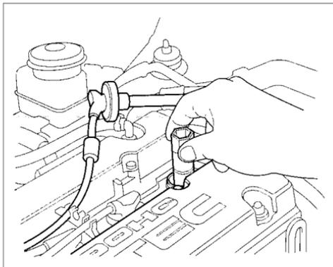
5. Put the new spark plug into the socket; then screw it into the hole. Screw it in by hand so you do not crossthread it.
