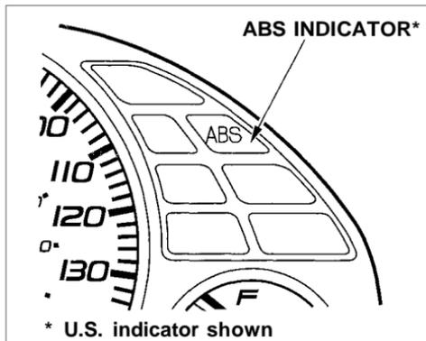
The ABS is self-checking. It also checks itself whenever you use the brakes.
