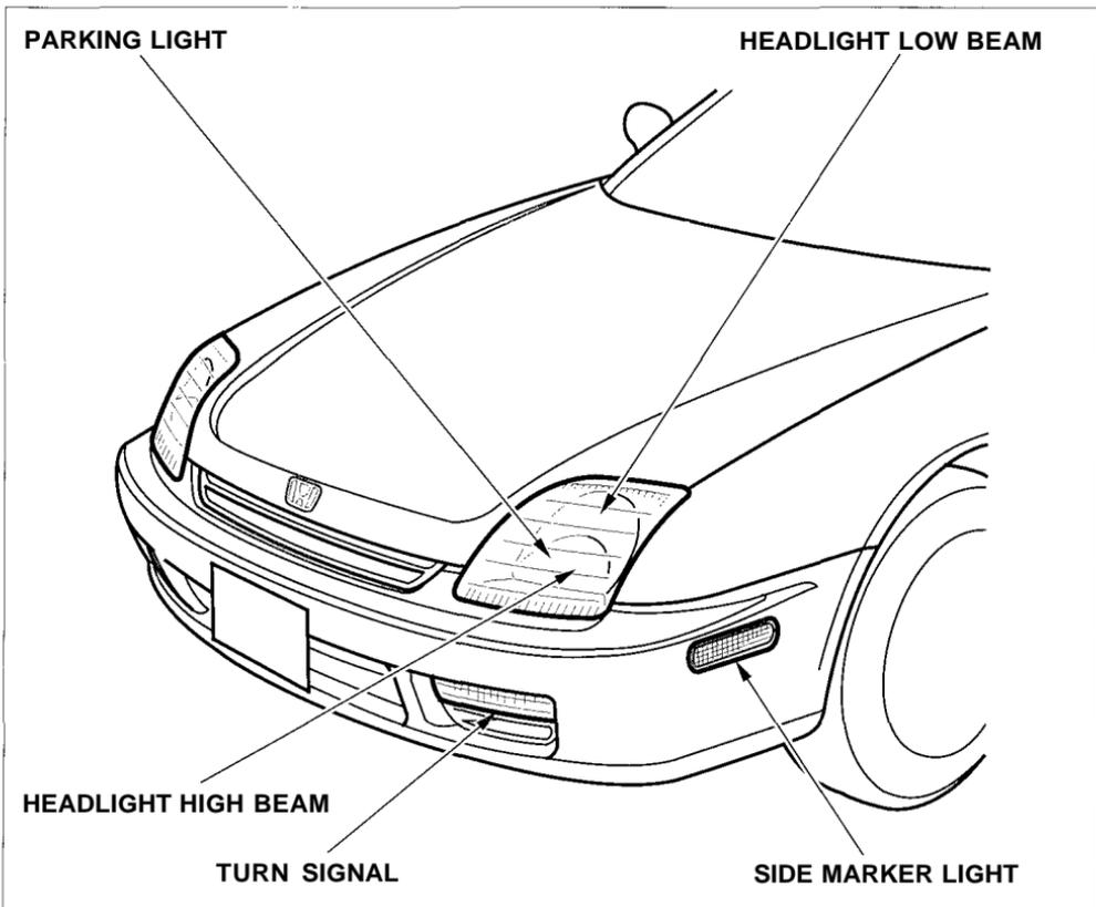
Check the operation of your vehicle's exterior lights at least once a month. A burned out bulb can create an unsafe condition by reducing your vehicle's visibility and the ability to signal your intentions to other drivers.
