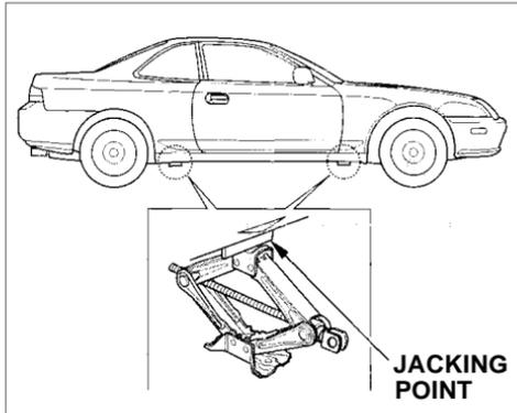
9. Locate the jacking point nearest the tire you need to change. It is pointed to by A mark molded into the underside of the body. Place the jack under the jacking point. Turn the end bracket clockwise until the top of the jack contacts the jacking point. Make sure the jacking point tab is resting in the jack notch.
