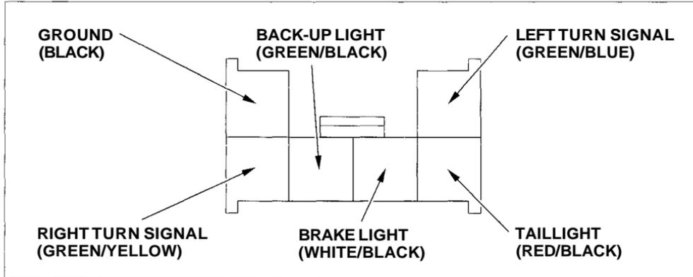
Your vehicle has a trailer lighting connector in the trunk by the left tail-light. To use the connector, undo the fastener on the left side of the trunk lining. Refer to the drawing above for the wiring color code and purpose of each connector pin.
