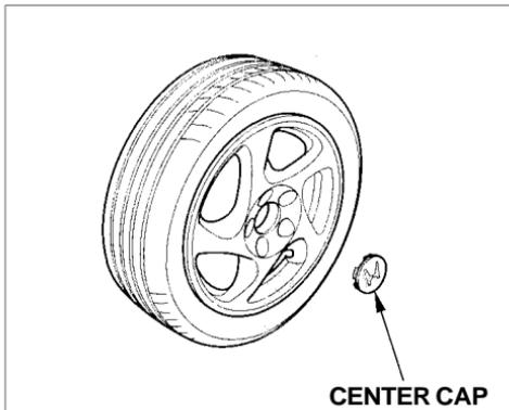
16. Remove the center cap before storing the flat tire in the trunk well.
