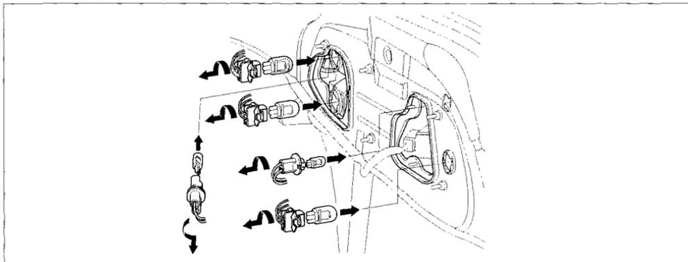
3. Determine which of the five bulbs is burned out: stop/taillight, turn signal light, side marker light, back-up light, or taillight.
