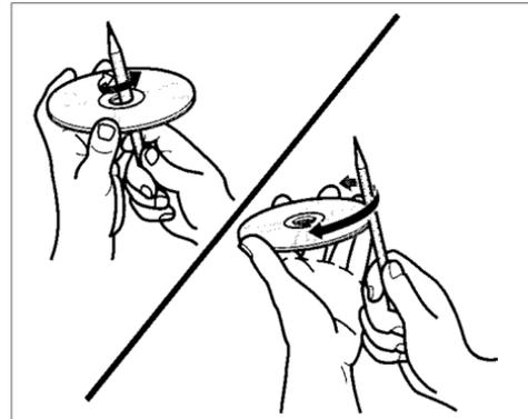
A new CD may be rough on the inner and outer edges. The small plastic pieces causing this roughness can flake off and fall on the recording surface of the disc, causing skipping or other problems. Remove these pieces by rubbing the inner and outer edges with the side of a pencil or pen.
