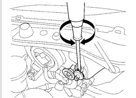
6. If either indicator is not aligned with its "0" mark as described, an adjustment can be made using a Phillips-head screwdriver to realign it with the "0" mark. Please refer to the illustrations.
