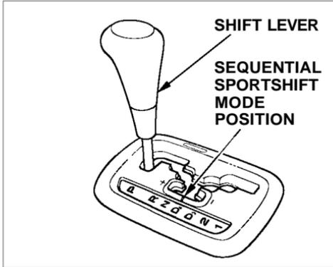
The shift lever has eight positions. It must be in Park or Neutral to start the engine. When you are stopped in D<sub>4</sub>, D<sub>3</sub>, 2, 1, N, R, or the Sequential SportShift mode, press firmly on the brake pedal and keep your foot off the accelerator pedal.
