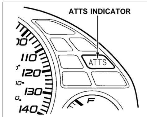
The Active Torque Transfer System (ATTS) is self-checking. If a problem is detected in the system, the ATTS indicator on the instrument panel comes on.
