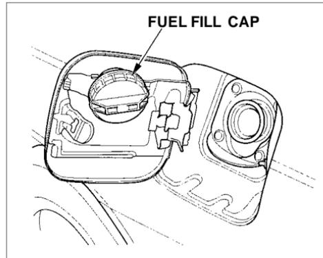
3. Remove the fuel fill cap slowly. You may hear a hissing sound as pressure inside the tank escapes. Place the cap in the holder on the fuel fill door.
