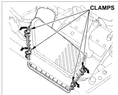
The air cleaner element is inside the air cleaner housing on the passenger's side of the engine compartment. To replace it:
