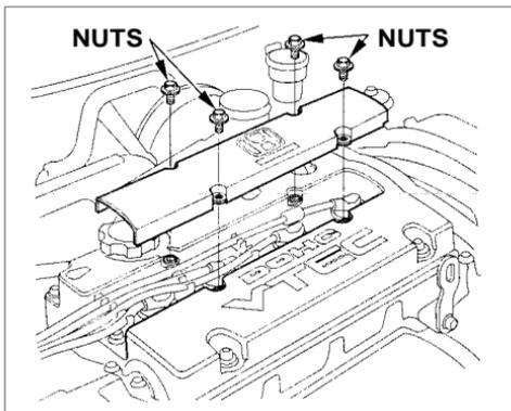
1. Remove the four nuts, then remove the plug wire cover.
