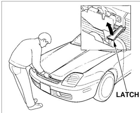
2. Standing in front of the vehicle, put your fingers under the front edge of the hood to the right of center. Slide your hand to the left until you feel the hood latch handle. Push this handle to the left until it releases the hood. Lift the hood.
